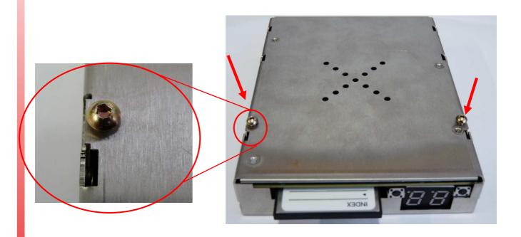
Step 2: Place the board on the emulator and slide the scsi board as seen below.
